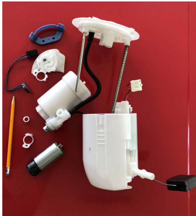
610. Figure 9 below depicts the component parts of a Denso fuel pump module.
